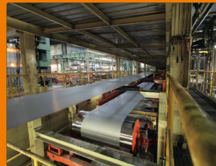
▲ A loop accumulator ensures continuous processing of the material.
