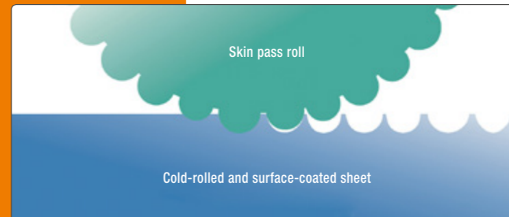
▲ Schematic representation of the process of applying the PRETEX® surface structure
