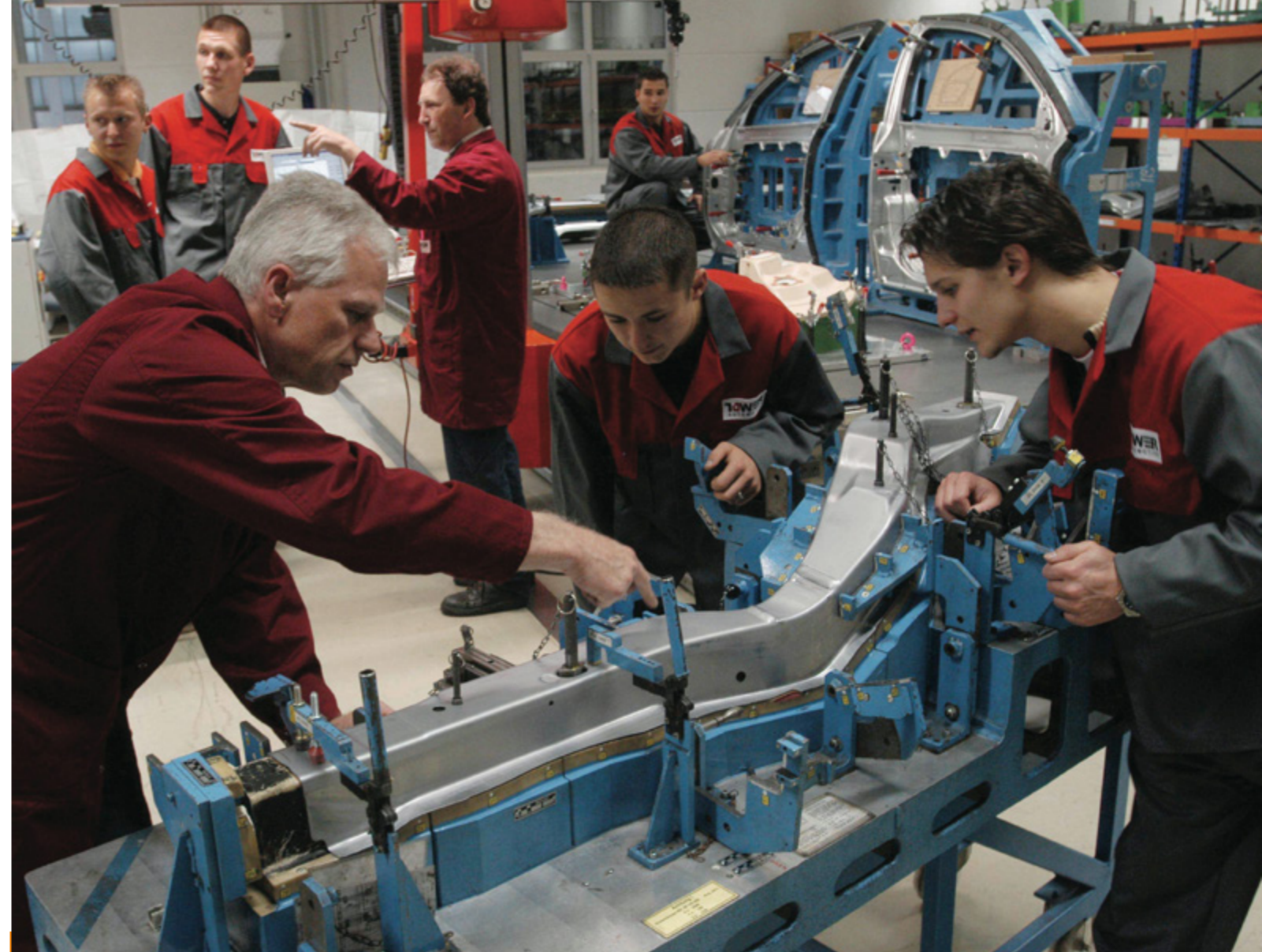
▲ Know-how right from the start: Trainees check a side member for the BMW X1 in the measuring room
